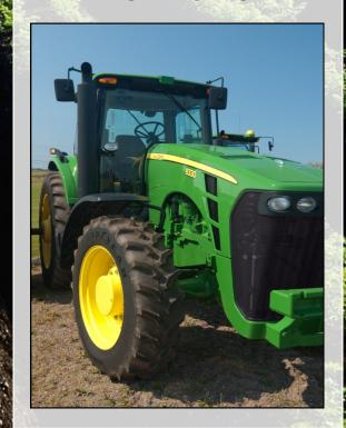
LIQUID BALLASTING IN TIRES HAS BEEN AN ALTERNATIVE TO CAST IRON WEIGHTS FOR MANY YEARS.
