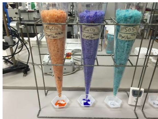
Figures 1 and 2: Imhoff cones filled with treated salt; Illustration of product leaching. (Treatment liquids dyed for visibility.)
