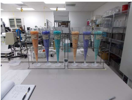
Figures 1 and 2: Imhoff cones filled with treated salt; Illustration of product leaching. (Treatment liquids dyed for visibility.)
