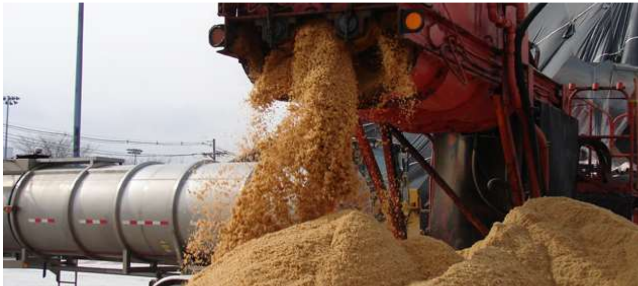
FIGURE 1: PUGMILL TREATMENT APPLICATION METHOD ON SAND
